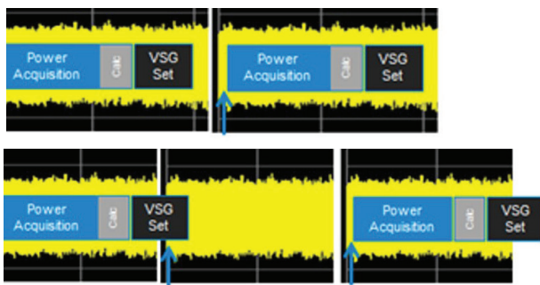
Figure 5. When optimizing a short waveform length, getting too aggressive can actually increase the test time if the waveform is made too short, as shown in the bottom graphic. Instead, the waveform should be set to just longer than the whole measurement cycle time, which includes the measurement time and processing time, as shown in the top graphic.
