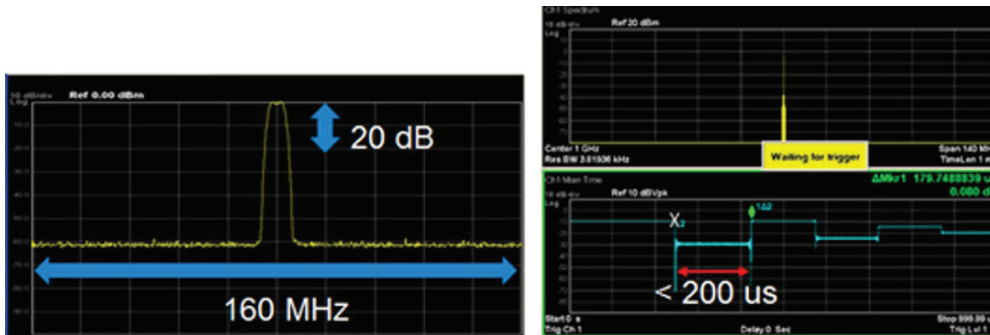
Figure 2. Using the power servo loop approach in the PXI VSG, amplitude changes can be achieved in less than 200 \mu s.
